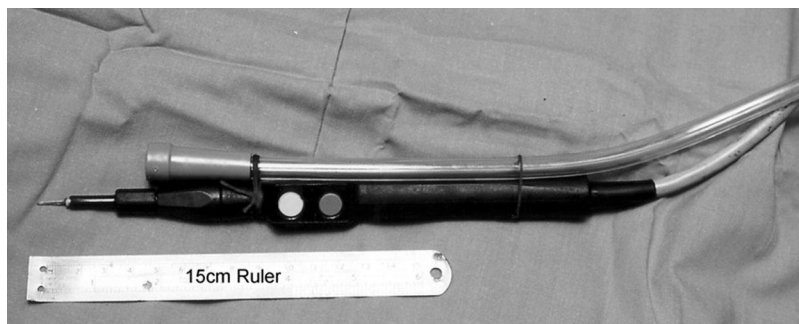
FIG. 1. A standard piece of silicone suction tubing with an internal diameter of 7 mm is secured to a handheld probe (from an ERBE APC 300 laser unit) using string ties. The open end of the tube is 5 cm from the laser tip and has a suction pressure of 30 kPa, to provide uptake of virtually all smoke plume in the operative field.
